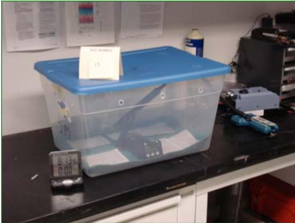
Note 6 heater packs, MSA Passport 5 Star instrument to monitor and log concentration of oxygen and carbon monoxide. The black cylinder sensor connects to the TSI IAQ Trak instrument outside the case; it logs concentrations of carbon dioxide, temperature and relative humidity. Cages were tested with and without a blanket cover. Cages modified with added ventilation openings were also tested by the same methods.
